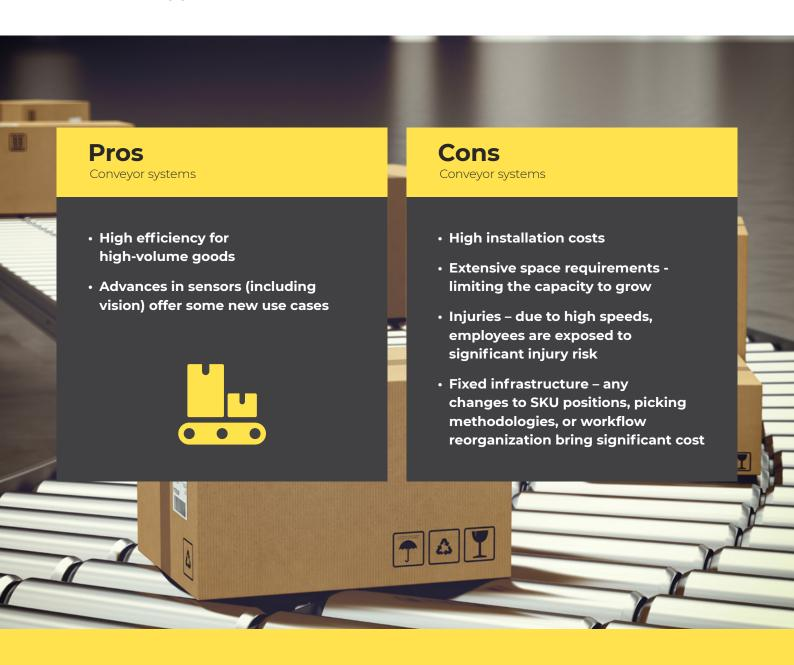
Conveyors are inflexible but efficient for handling high-volume goods with little seasonal fluctuations and for operations that don't expect significant changes to SKU positions or workflows.
