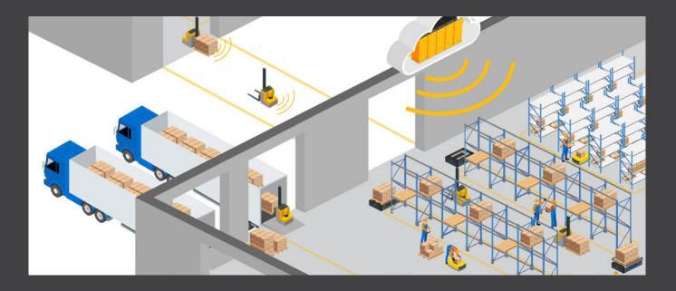
Autonomous mobile robots are a flexible tool that can adapt to dynamic and ever-changing facilities, where people and goods constantly move about. This superior adaptability minimizes infrastructure requirements, installation cost, and downtime when changes are needed. The most advanced solutions automate some historically manual operations for the first time, such as **trailer unloading** or **operating both indoors and outdoors**.
